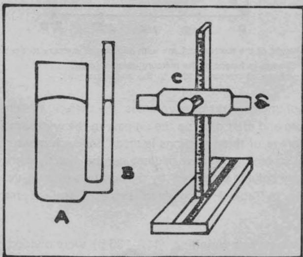
Fig. 1 : A schematic diagram of paw volume measuring apparatus.
